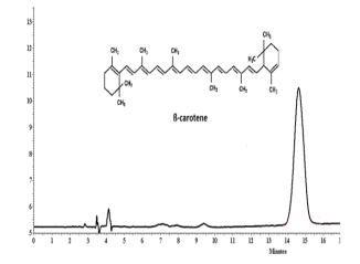
Figure 1. Representative chromatogram of  $\beta$ -carotene standard solution at  $\lambda$ = 453 nm. Chromatographic conditions: C18 column (ZORBAX 300 SB-C18 (4.6 x 250 mm x 5 $\mu$ ). Methanol/THF/Water; DAD detector (1260 DAD VL+)
